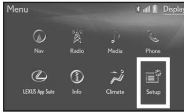
**STEP 2** Highlight "Setup" using the Remote Touch unit and push knob to select.
